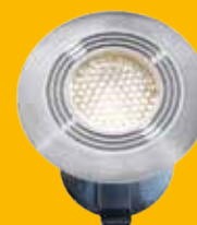
Onyx 30 R1 [150D] RVS 316 LED 0,5W 2.700K - 4lm 41 x 45 mm (HxØ) Boorgat: 30mm
